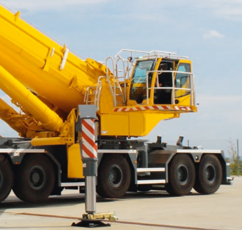
③ Self-assembly of the rear outriggers
