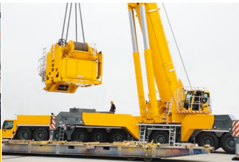
⑥ Self-assembly counterweight frame with drive assembly
