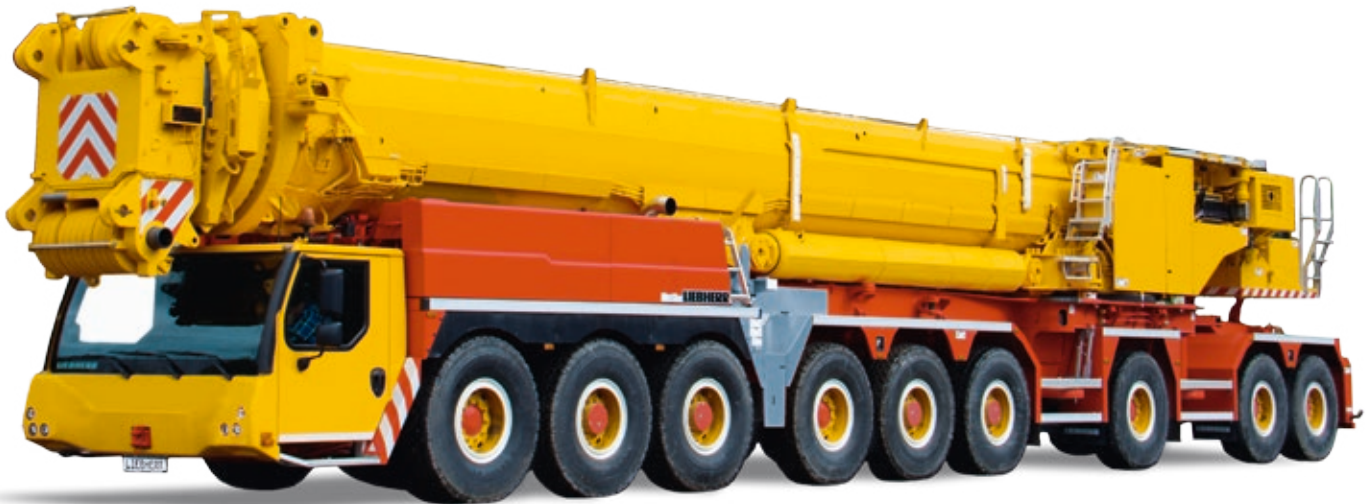
Total weight 99 t at 11 t axle load without outriggers
