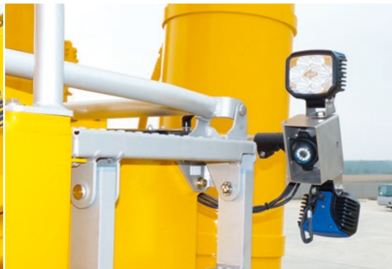
Camera monitoring of the slewing platform
