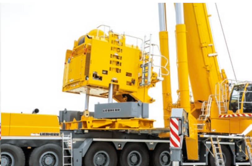
⑦ Cylinder of the counterweight frame fixed to the ballast ground plate
