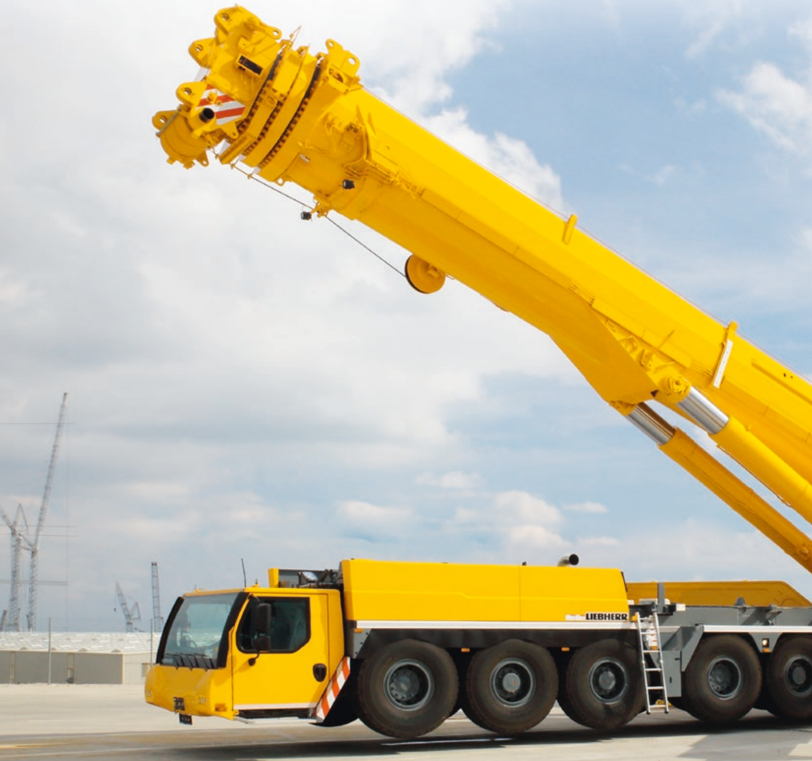
① LTM 1750-9.1 supported on the front outriggers
