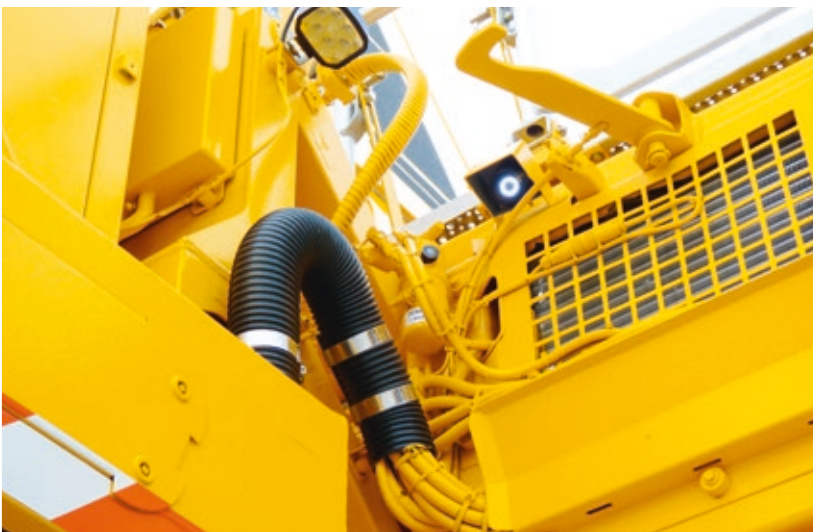
Camera monitoring of the rear of the crane cab
