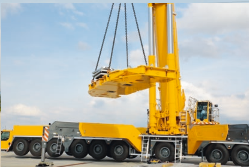
④ Self-assembly counterweight
