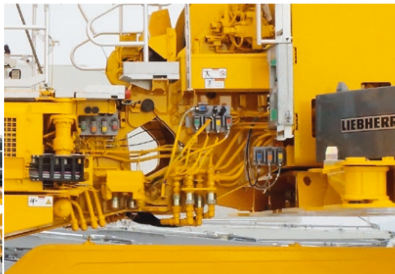
⑧ Connecting hydraulic and electric quick couplings
