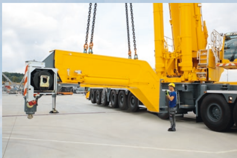
③ Self-assembly of the rear outriggers
